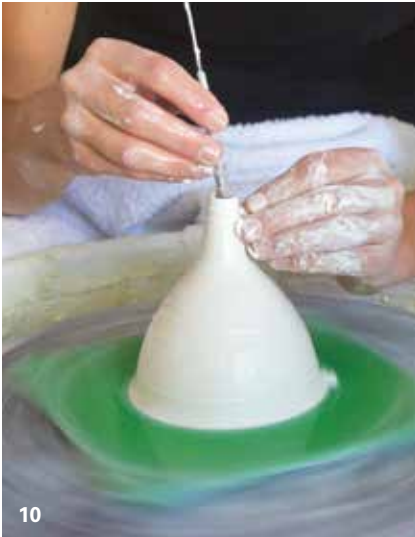
10 Throw a spout. Use the end of a needle tool to compress the tip of the spout.
