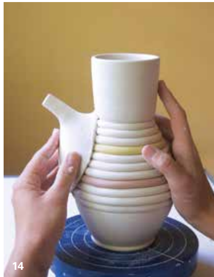
14 Score, slip, then gently compress the edges of the spout to the coils.
