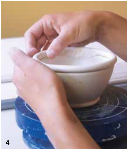
4 Use your thumb to compress the coil downward to the rim of the bowl.
