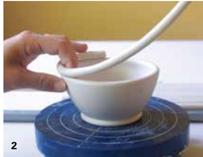
2 Add the coil to the rim using your other hand to guide its placement.
