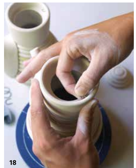
18 Push a piece of wire in the gallery, above the lid, opposite the spout, for a lid catch.
