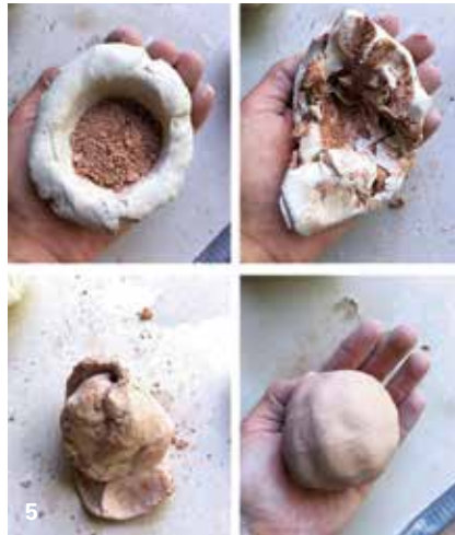
5 Hand wedge Mason stains into the porcelain with a small amount of water.
