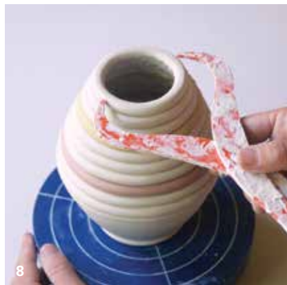
8 Measure the top of the coil form at its widest point with calipers.
