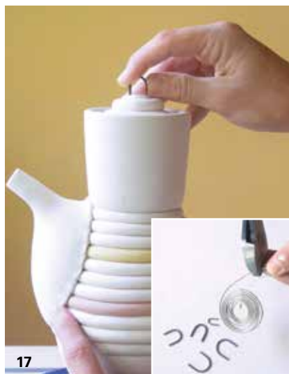
17 Push two pieces of nichrome wire, side-by-side, into the center of the lid.
